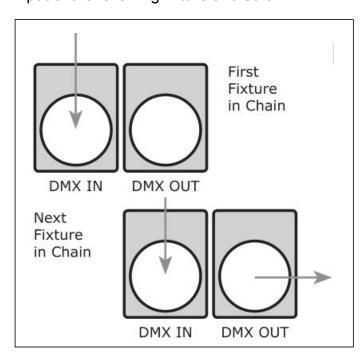
A quick note: Often, the setup for Master-Slave and Standalone operation requires that the first fixture in the chain be initialized for this purpose via either settings in the control panel or DIP-switches. Secondarily ,the fixtures that follow may also require a slave setting.
